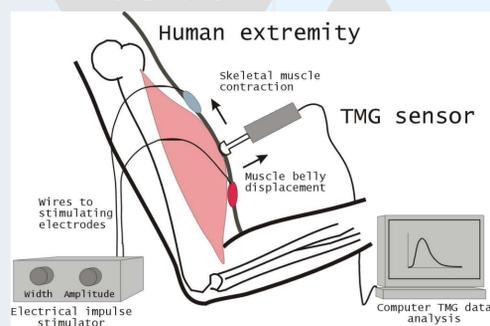
Figure 1. Assessment using Tensiomyography
